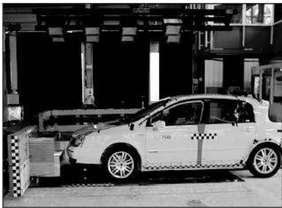
Fig.9.1; Test de impact frontal, EuroNCAP (European New Car Assessment Programme-Program de Evaluare al Vehiculelor Noi).
