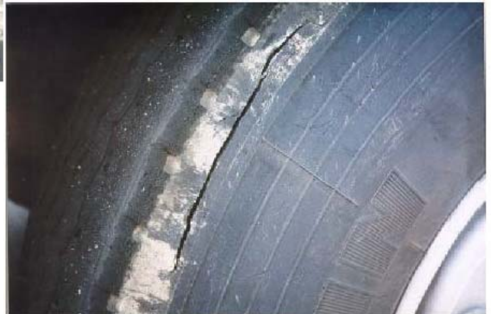
Fig. 2.5: Tyre damage (e.g. cracks or cuts in sidewall) illustrated by a truck tyre
