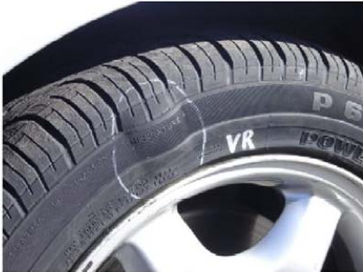
Fig. 2.7: Tyre damage (e.g. buckles in sidewall)
