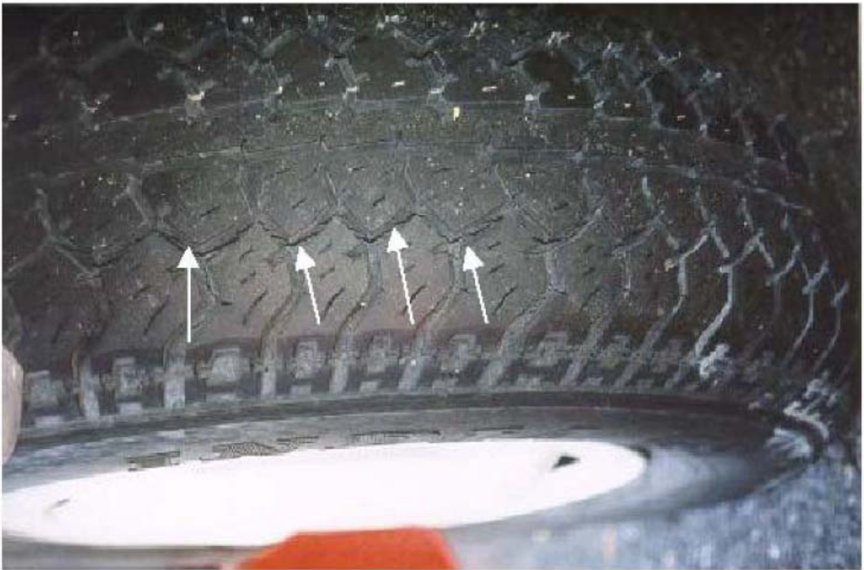
Fig. 2.6: Aging defects (e.g. cracks)
